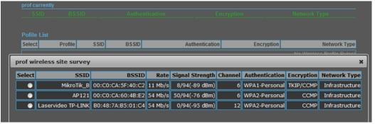
3) Now, it shows the Profile Name, SSID, BSSID, and encryption type received from your target network and press **Next** button to finish the wizard.
