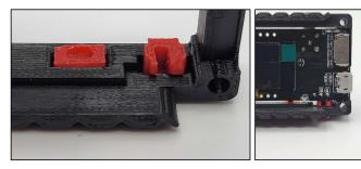
Installing the reset button (left) and power switch (right) Note: install both before inserting LoRa board
