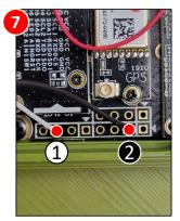
Solder the other ends of these two wires to the IO.2 (1) and GND (2) pins on the RAK19007/5005 base board
