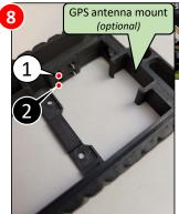
RIGHT TWO (on the same side) legs of the user button, then solder the other ends of these two wires to the AIN1 and GND pins on the RAK19007/5005 base board as shown above (GND can be shared with wire from step #7)
