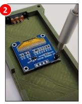
Mount the 0.96" OLED screen and secure with four M2x4mm screws & washers (disregard if no screen will be installed)
