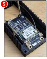
Install the RAK19007/5005 board using four M2x4mm screws & four M2 nuts
