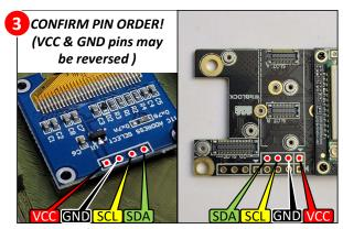
**Solder four wires** to the screen I2C pins, then **solder the other ends** of these four wires to the RAK19007/5005 base board as shown above
