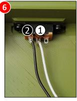
**Solder two wires** to the **LEFT TWO** contacts of the GPS switch
