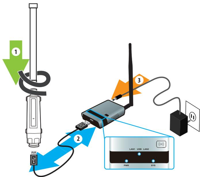
1. Mount the antenna AOA-2409TF to Tube-U(N) securely, and seal the gap on the N-type connector with weather-resistant tape.
